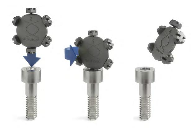
Up to six plugs can be assembled on a handling aid. This allows a simple installation without any tools. The handling aid inserts the plug into the screw recess. The handling aid is then rotated or tilted to release the plug. Once it is inserted, the PARRYPLUG® immediately provides efficient protection against unauthorised access. Quick and simple: The installation operation can be repeated without any further preparation until all of the plugs are installed.
