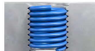
Correct installation of the HELICOIL® Smart (0.25–0.5 x P below the component surface)
