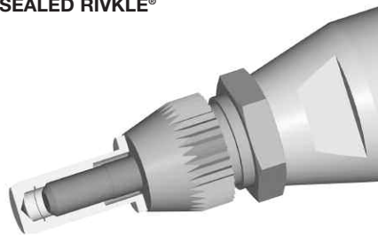
Thread root single-turn rod
