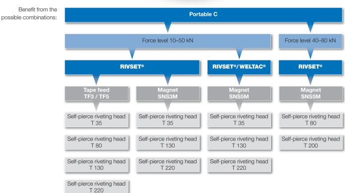
T = throat, TF = tape feed, SNS3M = self-pierce riveting punch with magnet for 3-mm rivets, SNS5M = self-pierce riveting punch with magnet for 5-mm rivets and  $WELTAC^{\circledcirc}$  elements
