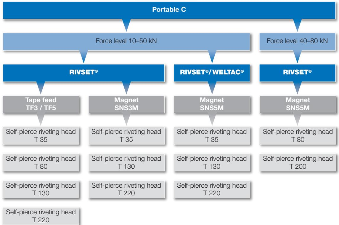
T = throat, TF = tape feed, SNS3M = self-pierce riveting punch with magnet for 3-mm rivets, SNS5M = self-pierce riveting punch with magnet for 5-mm rivets and WELTAC® elements
