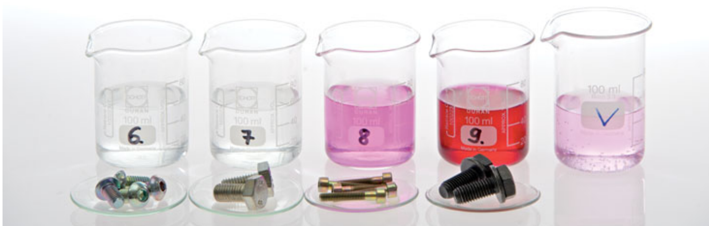
Laboratory testing for the determination of Cr 6+ in anti-corrosion coatings
