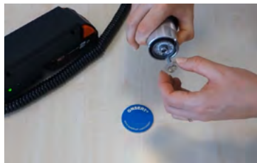
Insertion of the ONSERT® fastener into the tool holder
