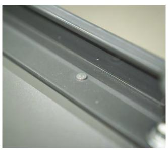
High-strength joint with RIVSET® self-pierce rivets
