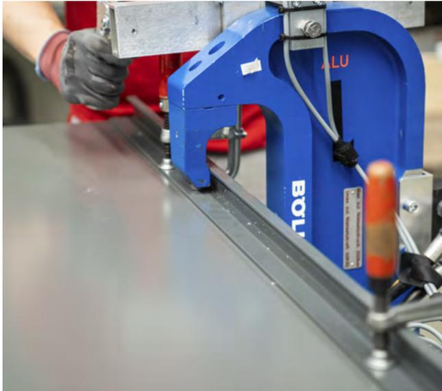
RIVSET® "Roadsign": robust and flexible self-pierce riveting system for modern sign manufacturing
