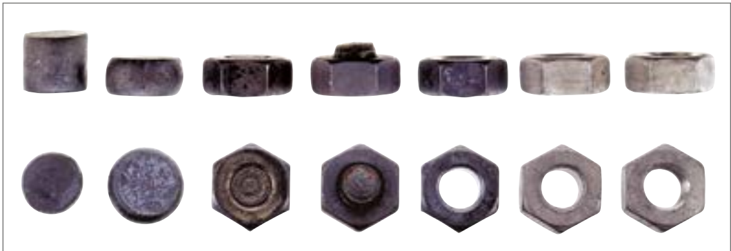
Figure 5.4 Forming stages of a hexagon nut
