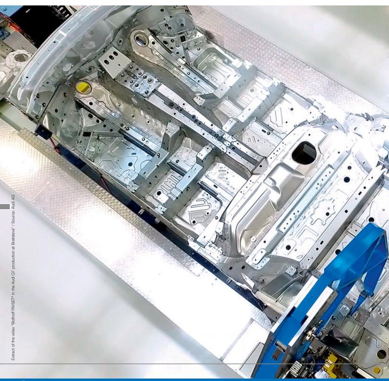
The main requirements for this system are a 100% electrical installation on robots, the compact design of setting tools and short process times, for some applications < 1.5 s.
