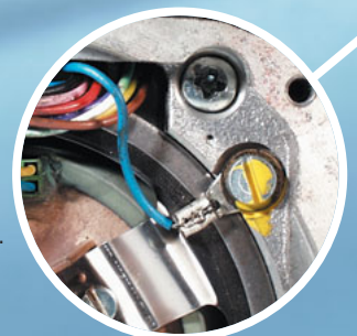
Controller. Three-phase servo motor with electronic positioning unit. Loose tangs would result in faults.
