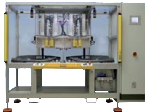
Special thermal installation machine for the simultaneous embedding of six HITCERT® thread inserts in two car door trims
