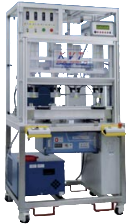
ERW thermal installation machine for embedding four HITCERT® thread inserts in a boot handle
