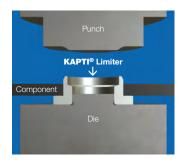
The KAPTI® Limiter and the plastic component are positioned on the die of the riveting tool.
