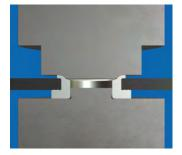
Flanging the end of the shaft to create a form-fit joint between the KAPTI® Limiter and the component. Forming the sealing lips into the plastic.
