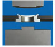
Retracting the stamp and removal of the composite from the KAPTI® Limiter and the component.
