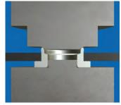
Closing the tool and placing the punch on the shaft end of the KAPTI® Limiter. Start of the forming process.
