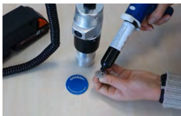
Application of the adhesive to the ONsert® fastener
